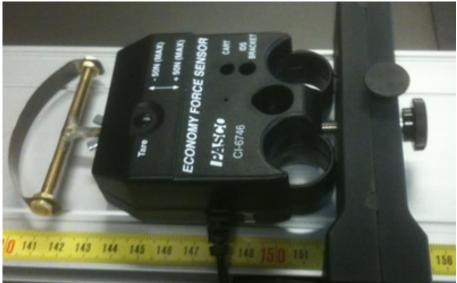
You will, of course, need to tighten the screw so the Force Sensor is firmly mounted. Now the Force Sensor will measure the force exerted on it by the Cart. How is this related to the force exerted by the Force Sensor on the Cart?
